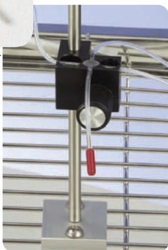
MCLA/GC Counter-balanced lever arm for swivel with pocket to hold 4-way connector
