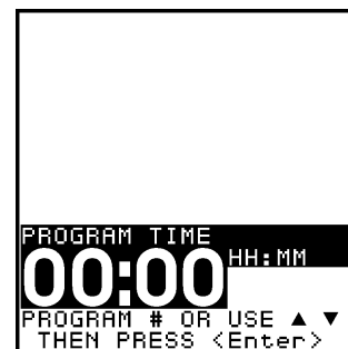
Figure 8.2.3: Setting Stand-By Timer
