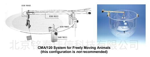
**Problem.** The design of the CMA balance arm allows movement of the swivel in one axis only, which places stress on the swivel and may result in failures. In the case of the 375/D/22QE swivel, the most common failure mode is an unintended unscrewing of the swivel cap during operation. Instech's newer 375/D/22QM<sup>†</sup> model may actually break under these stresses.
