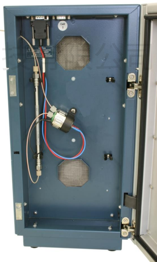
Fig 3. Left : SenCell with ISAAC reference mounted in DECADE II detector. [1] Cell clamp, [2] Cell Inlet (tubing connection from column-to-cell), [3] Cell outlet (tubing connection from cell-to-waste), [4] WE contact (red), [5] AUX contact (blue), [6] REF contact (black). Top-right : electrical connections of WE (red connector) and AUX electrode (blue connector). Bottom-right : SenCell with Saltbridge reference electrode.
