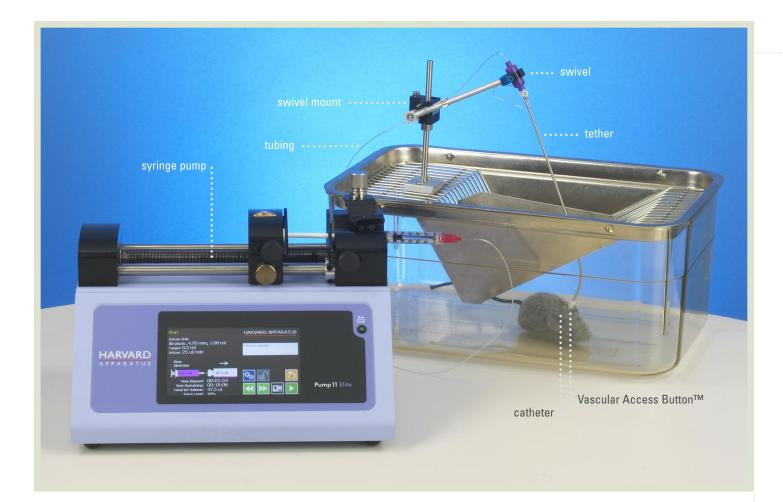
Choose your equipment carefully when setting up continuous mouse infusion studies. A typical mouse can turn a swivel with no more than 0.025oz-in of frictional torque. Instech has three models that meet this specification: a 25ga stainless steel model, a 25ga plastic model, and the 375/D/22LT dual channel model. Always use a spring counter-balanced lever arm to remove the weight of the tether from the mouse.
