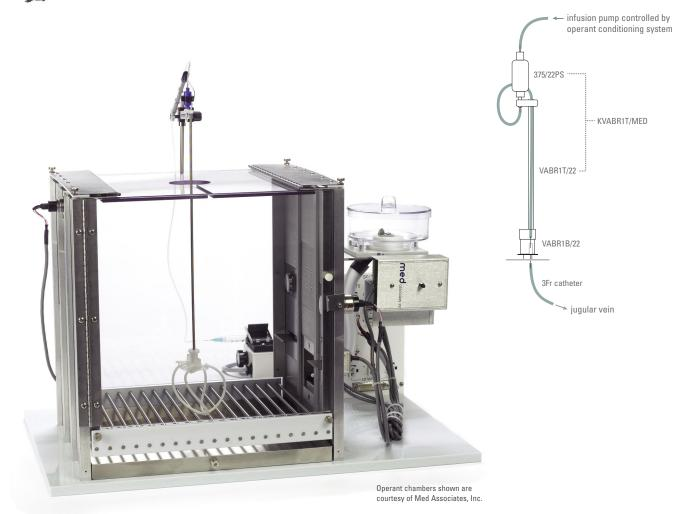
Instech swivels, tethers and balance arms are used with operant behavior systems for IV self administration studies. A lever press or nose poke will trigger an IV dose from a syringe pump.
